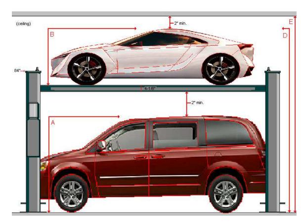
Next, the lift will have a maximum clearance underneath of 70" on the 8000 model and 77" on the 8000XLT model when resting on the highest safety lock position. The vehicle you park underneath must be lower than 70" to use the 8000 model or 77" for the XLT model. The vehicle you park on top must be lower than your ceiling height less 74" for the 8000 or 81" for the 8000XLT. (Also, consider the location of your garage door when open and garage door opener if you have one.)
